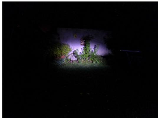
Figure 4: High beam of a 6W "LD" LED bulb in a BSA C11 lamp.
