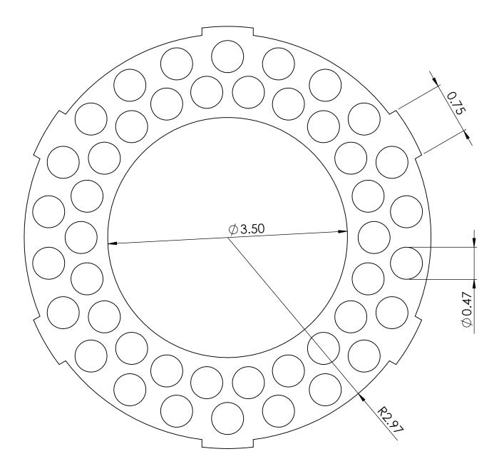
Clutch Friction Plate with 44 holes for cork inserts
