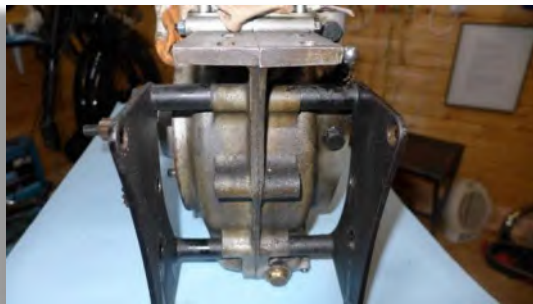
Figure 31: The crankcase on the bench (working plate). The rear carrier plates are still attached.
