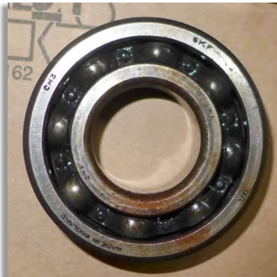
Figure 44: The RLS8 ball bearing on the driving side.
