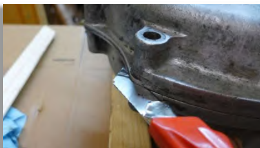
Figure 33: Opening the crankcase. Like for the timing cover one should not apply force but the careful use of a cutter blade to avoid damage.
