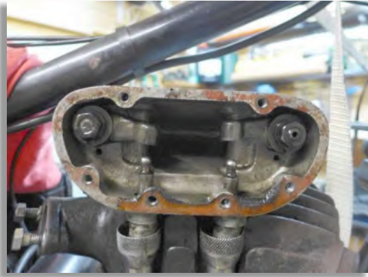
Figure 6: The rocker box on top of the cylinder head. Note the cups for the pushrods at the rocker arm ends. The rocker box cannot be shifted aside until the pushrods are lowered.
