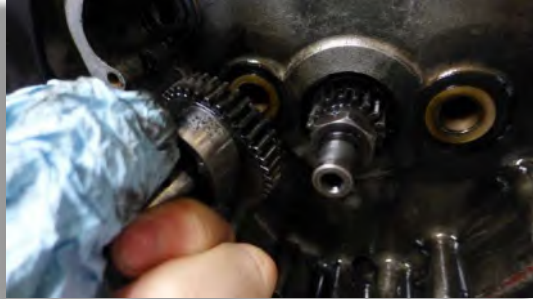
Figure 13: Since the camshaft positions are unambiguously referenced by marks the shafts can be pulled out of their bushes.
