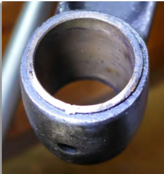
Figure 42: The small end phosphor bronze bush in good condition.
