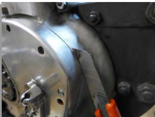
Figure 2: Opening the timing cover. To avoid damage, one should not apply force but the careful use of a cutter blade and a hammer.
