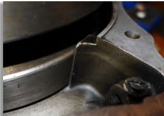
Figure 36: The blade of the oil separator on the timing side next to the hole for the oil drain plug with its filter.
