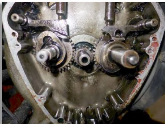
Figure 4: Contents of the timing cover with the two camshafts and their respective rocker arms. Note the moveable inner part of the exhaust cam shaft for the valve lifter.
