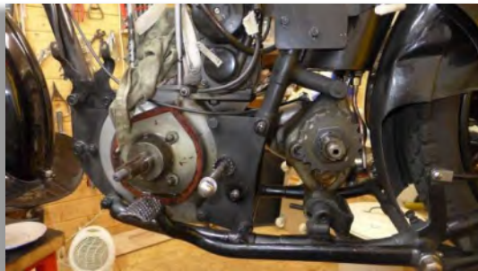
Figure 22: Side view after the primary chain case is dismantled. Note the gasket on the left crankcase which has to be renewed.
