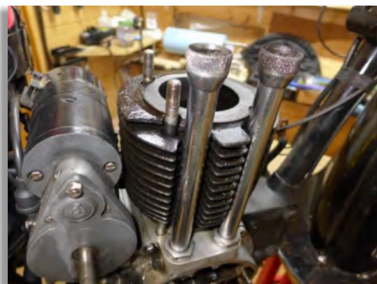
Figure 11: The Sunbeam has no cylinder head gasket and the surfaces must not be damaged.
