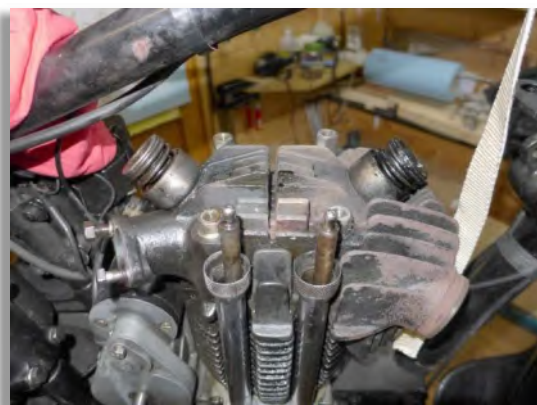
Figure 8: The cylinder head without the rocker box.
