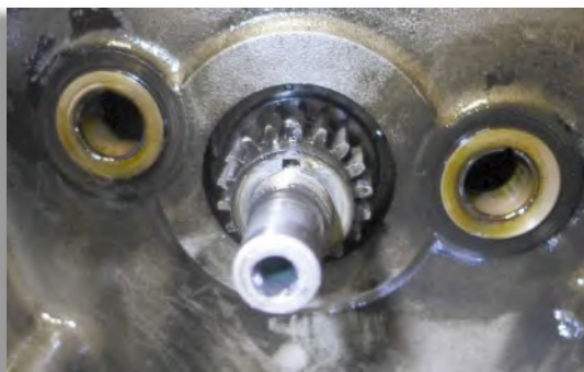
Figure 41: The two plain bearings of the lower rocker arms in the timing case.
