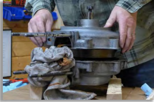
Figure 34: As soon as the two crankcase halves are loose one can carefully separate them from each other.
