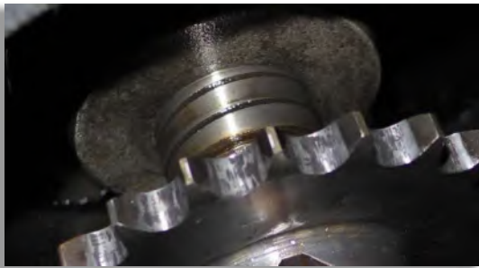
Figure 17: When pulling off the drive sprocket the oil scroll dynamic seal with its worm grooves becomes visible. The seal rotates counterclockwise and the grooves transport leaking oil back into the crankcase.
