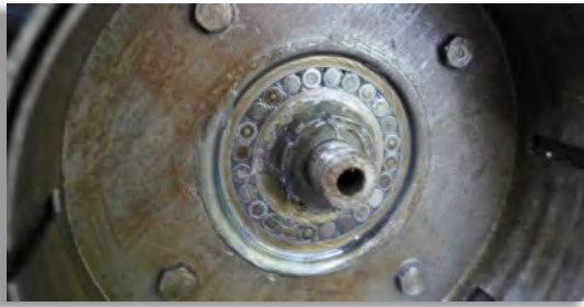
Figure 20: The clutch rollers inside their housing. The rollers are not positioned in a cage but are freely moving in a housing consisting of a front and back thrust washer and the inner and outer race (here well lubricated). When the outer cage is pulled out, all rollers will fall out.
