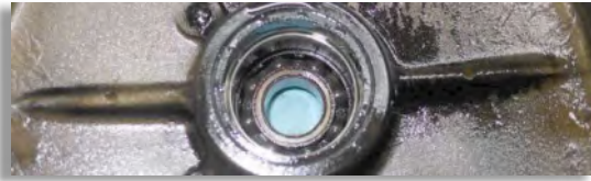
Figure 38: The crankcase driving side. On the outer side is an imperial RLS8 ball bearing of 2 ¼ inch outer diameter, 1 inch shaft diameter and 5/8 inch width.
