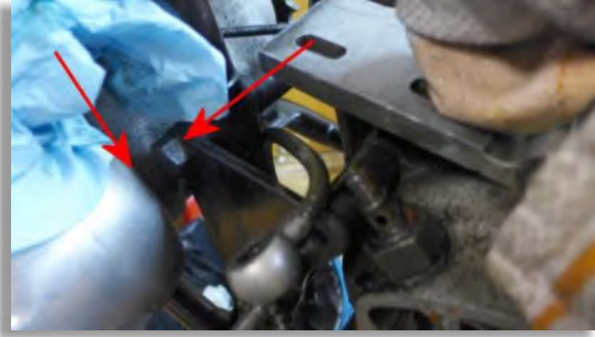
Figure 28: The upper rear bolt of the two carrier plates cannot be pulled out in its regular position. The gearbox is in the way and must be pushed aside.
