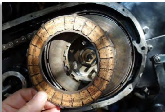
Figure 19: Dismantling the clutch.
