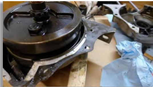
Figure 35: The old 0.35 mm gasket between the two halves of the crankcase.
