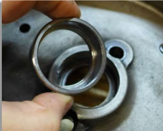
Figure 45: The RMC22L race. Note the lip on the race which avoids axial shaft movement.
