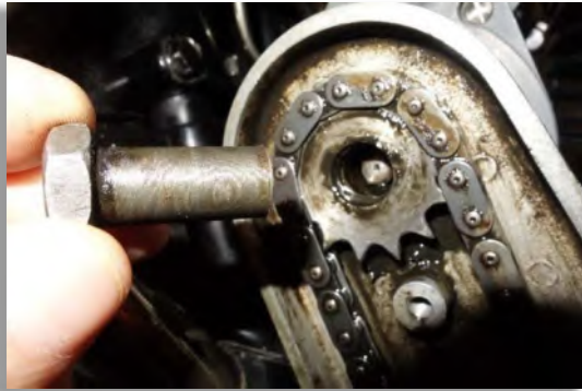
Figure 1: The upper sprocket pulled off the magneto taper.
