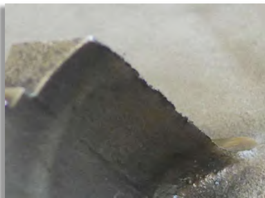
Figure 37: The blade of the oil separator on the driving side. Note the damage at the blade edge.
