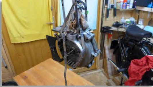
Figure 30: The crankcase is lifted out of the frame, the motorcycle on the trolley pushed beside and the case is then lifted onto a bench (working plate).
