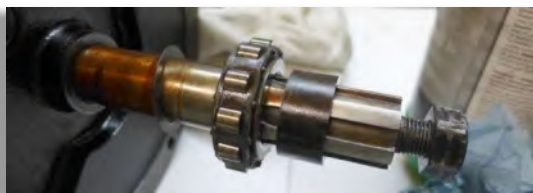
Figure 39: The imperial timing side LRJ1L (alternatively CRL8) roller bearing on the crankshaft driving side. Note that the LRJ series represents various bearings of different size and designs. The bearing for the Sunbeam must have a lip to avoid axial shaft movement. There are shims on both bearing sides. They are for adjusting the shaft end float.
