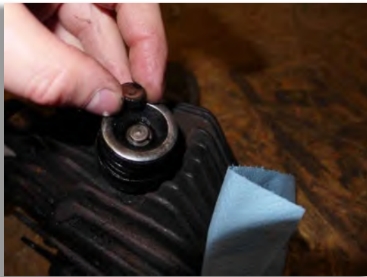
Figure 10: Hardened cups protect the valve tips against wear.
