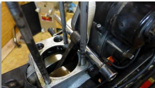
Figure 18: The conrod in the flywheel inside the crankcase. (To unlock the nuts on the crankshafts a bolt should not be positioned into the small end unless great care is taken not to mark the bearing face.)
