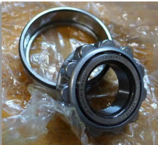
Figure 43: The imperial timing side LRJ1L (alternatively CRL8) roller bearing on the crankshaft driving side. Note that the LRJ series represents various bearings of different size and designs. The bearing for the Sunbeam must have a lip to avoid axial shaft movement. There are shims on both bearing sides. They are for adjusting the shaft end float.
