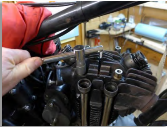
Figure 9: Diametric loosening the bolts of the cylinder head.
