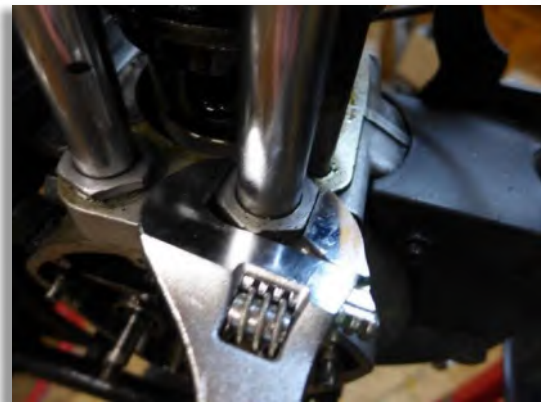
Figure 12: The push rod tubes are screwed into the crankcase but not into the rocker box.
