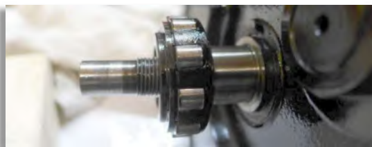
Figure 40: The metric timing side RMC22L roller bearing on the crankshaft timing side (‘L’ indicates a lip on the bearing race). It is a metric bearing of 50mm outer diameter, 22mm shaft diameter and 17mm width.
