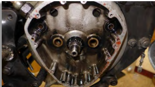
Figure 14: The timing case is cleared of its parts. The small hole at the lowest end acts as an oil pipe from the sump to the timing case and then to the oil pump. The central crankshaft is hollow. It acts as an oil pipe to the con rod big end. On the upper left side is the connection to the vent pipe.
