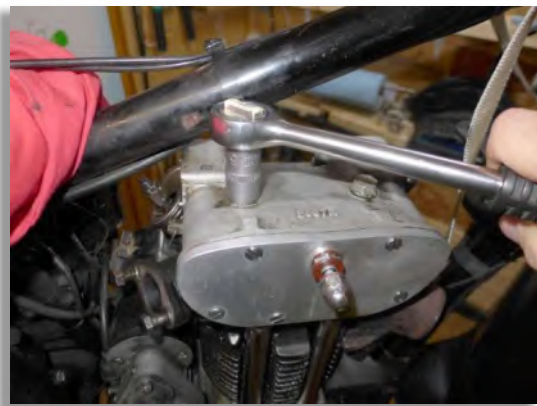
Figure 7: Loosen the bolts of the rocker box.
