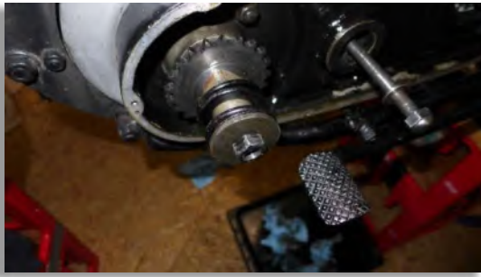
Figure 16: The cush drive inside the primary chain case. The central nut is locked by an already removed cotter pin.
