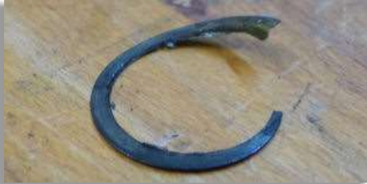
Figure 48: The compressed and torn shim on the inner side of the timing roller bearing.
