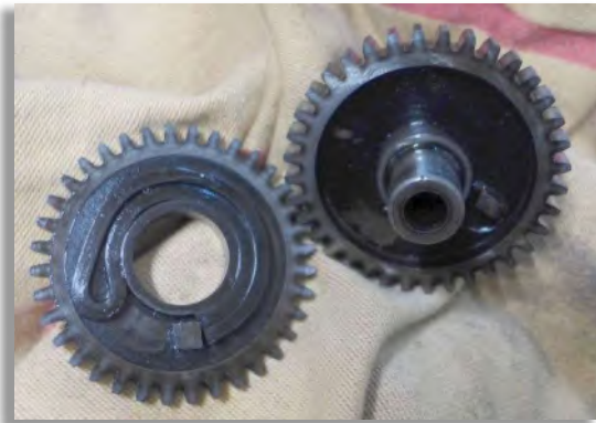
Figure 64: An open camshaft with the internal spring mechanism.
