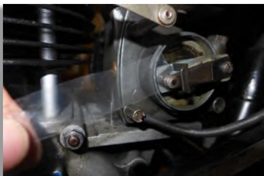
Figure 88: Cellophane sheet between the magneto points. As soon as the points open one can pull out the sheet.
