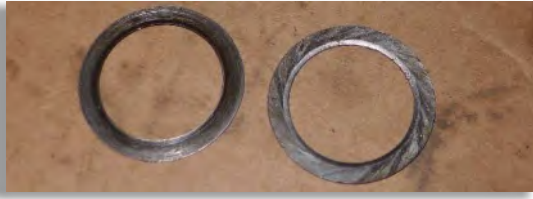
Figure 47: One shim was installed on each side of the main roller bearing for end float adjustment. The thicknesses here are 0.014" (0.365mm) and 0.015" (0.385mm).
