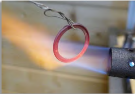
Figure 81: Annealing the copper gasket of the pushrod tube.
