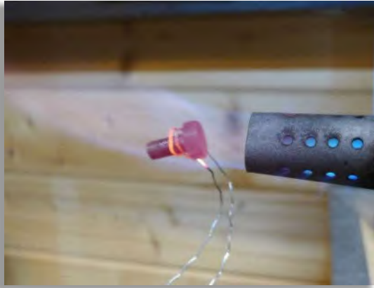
Figure 101: Heating a bolt for blueing it.
