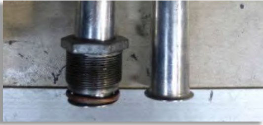
Figure 80: The bases of the two pushrod tubes. Left with its respective gasket-sealed connector to the crankcase.
