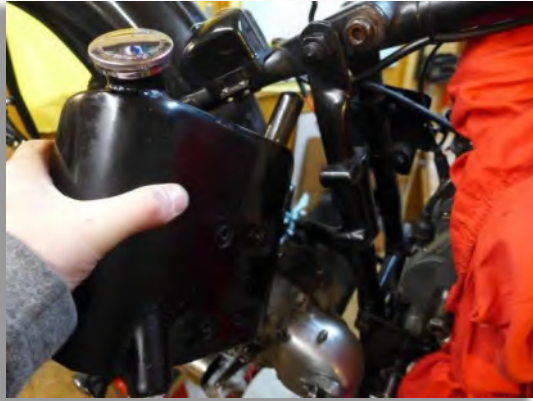
Figure 66: After loosening the four tank mounting bolts, the tank can be pulled out to the side.
