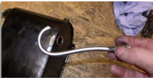
Figure 68: The oil return plug with its pipe.
