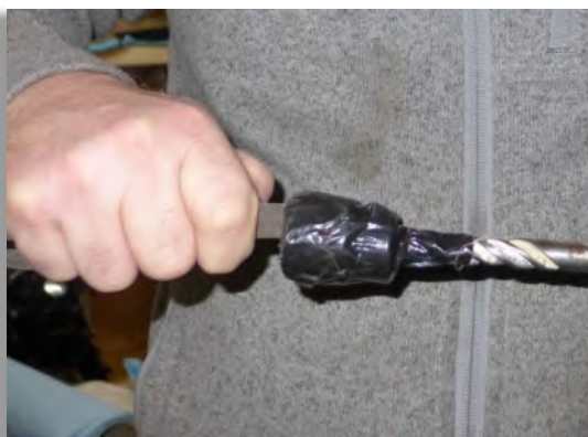
Figure 50: At high revs, the inner diameter of the shim is enlarged with a half-round file.
