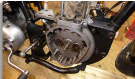
Figure 60: The crankcase back in the frame.
