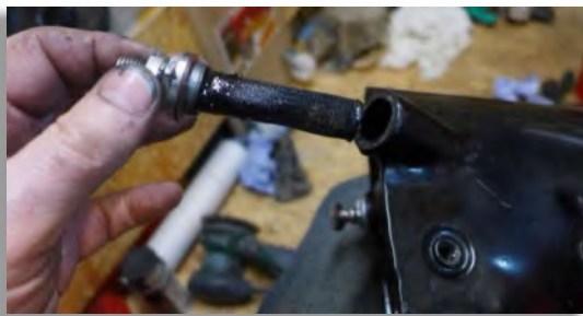
Figure 67: The oil feed plug with a mesh filter.
