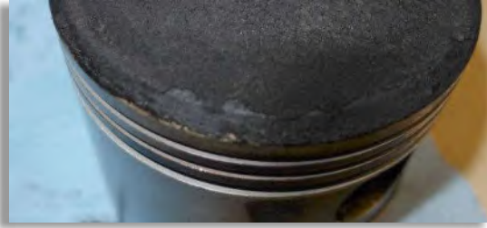
Figure 72: A strongly carbonized piston.
