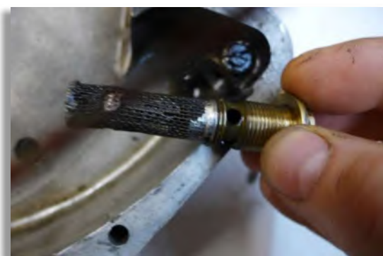
Figure 103: The old damaged sump oil filter.
