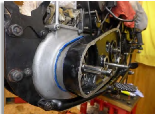
Figure 62: Assembly of the inner primary chain case.
