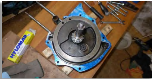
Figure 56: The crankcase just before being closed.
