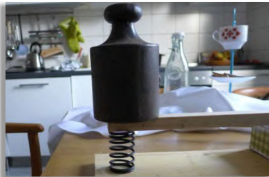
Figure 93: Measuring the spring constant with a market weight.
