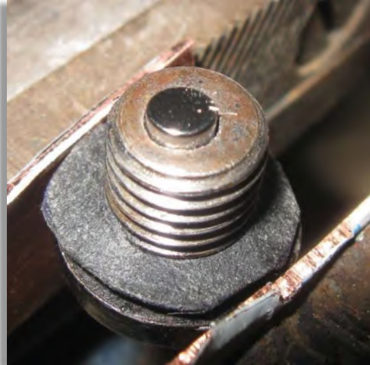
Figure 70: A Neodymium magnet in the oil plug.
