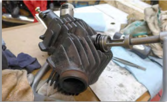
Figure 89: Removing the valves with a suitable tool.
