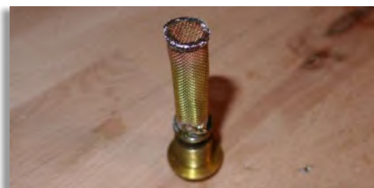
Figure 104: The soldered brass filter with a smaller mesh width.
