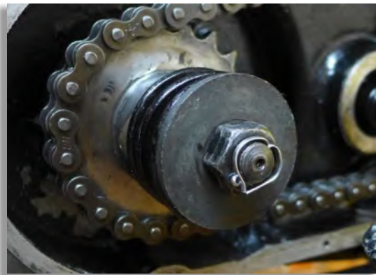
Figure 98: The cush drive is secured with a new cotter pin.
