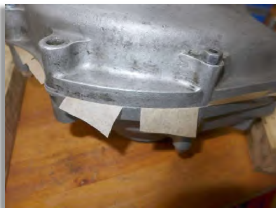
Figure 53: Testing for the correct end float with 2 thou backing paper.
