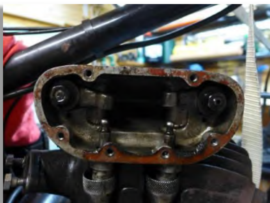
Figure 84: The upper rocker box between upper frame tube and cylinder head. Note the two pushrods intruding the box.
