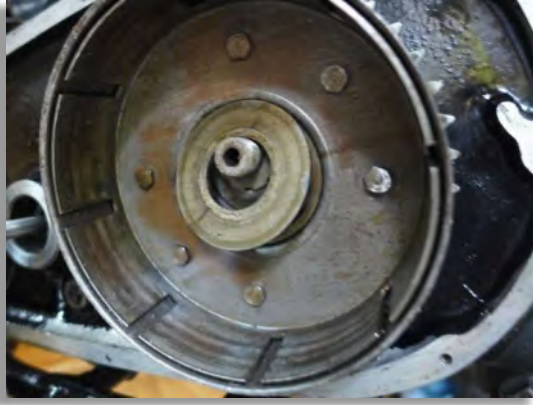
Figure 63: The loose front washer inside the clutch which covers its roller bearing. The respective back washer has a larger thickness.
