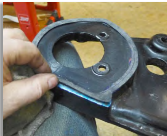
Figure 61: The new gasket between the crankcase and the inner primary chain case is embedded in Hylomar.
