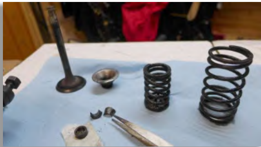
Figure 90: The dismantled valve components. Note the two collets which hold the valve in the spring via the cone dish.
