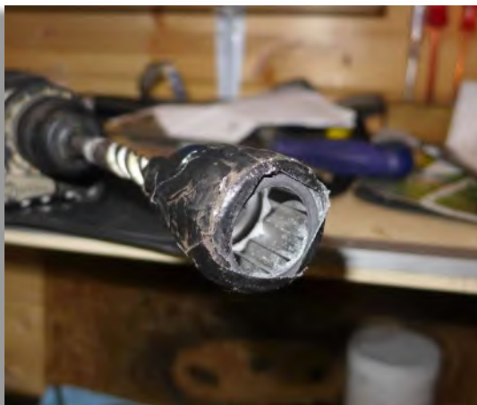
Figure 49: A shim fixed to a hexagonal nut with adhesive tape.
