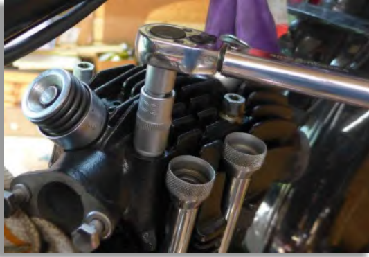
Figure 95: The 7/16 inch bolts are carefully tightened crosswise with a torque wrench.
