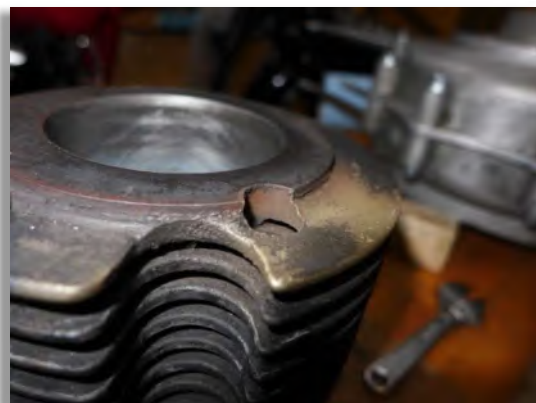
Figure 75: A bronze cylinder surface appeared after using a brass brush for cleaning the fins.
