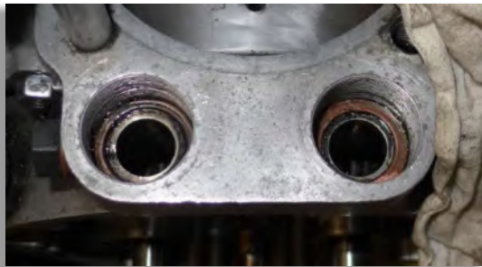
Figure 82: The copper gaskets in the holes for the pushrod tube connectors. They are left untouched because they are pressed firmly into their seats.
