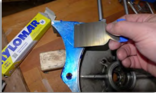
Figure 55: Applying the non-hardening jointing compound Hylomar M to the two crankcase parts.
