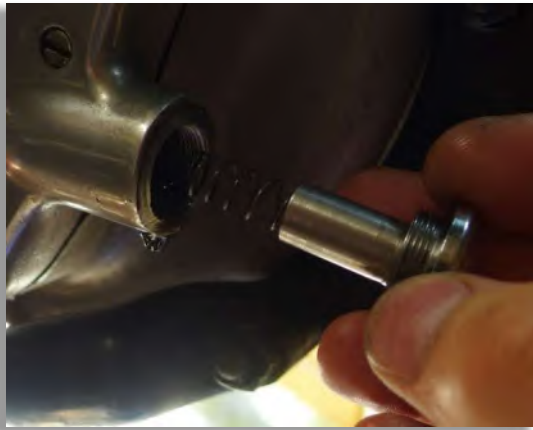
Figure 99: The screw and spring of the ball valve.
