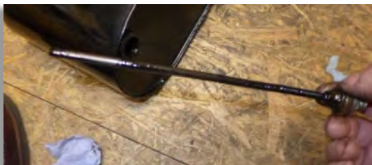
Figure 69: The tank breather plug with its straight pipe.
