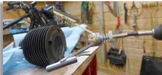
Figure 74. A cheap honing tool breaks the glaze with its three grinding heads.
