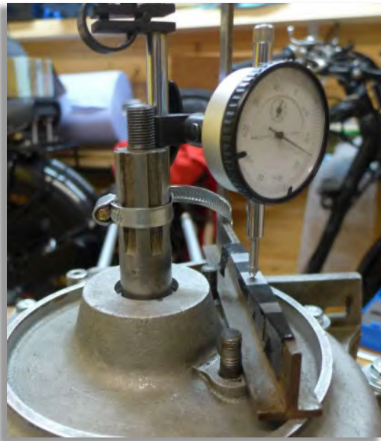
Figure 51: The gauge attached to the shaft.
