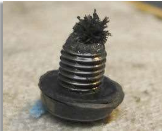
Figure 71: Metal chips on the magnet of the oil drain plug.
