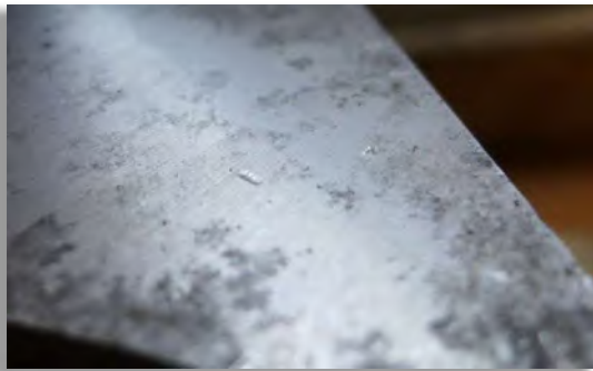
Figure 54: Part of the crankcase sealing surfaces. It represents the most disturbed part. The other surface parts look better.
